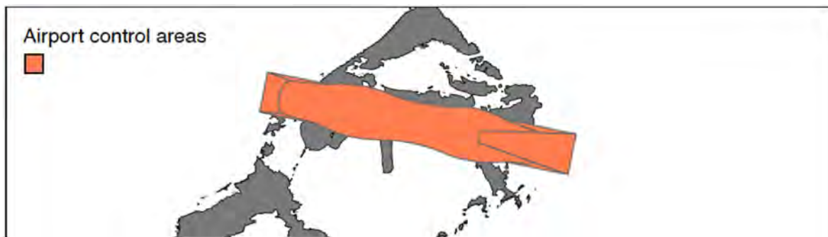
Figure 8.3.9. Exclusionary criteria were used to identify potential areas for renewable energy siting. This map shows the airport control areas (in orange), which are assumed to be unsuitable for wind energy platform siting.
